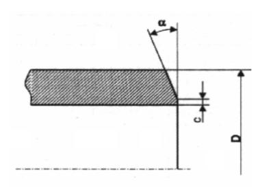
Figure 1 — Tube end bevel
