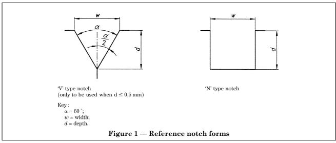
**4.6** The reference notch shall be formed by machining, spark erosion or other methods.
