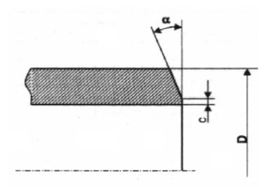
Figure 1 — Tube end bevel
