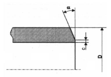
Figure 1 — Tube end bevel
