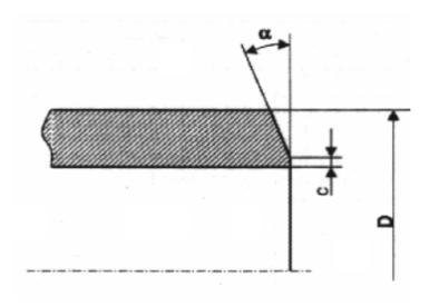
Figure 1 — Tube end bevel
