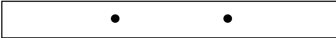
Example 1: Two 1/8 in. (3.2 mm) discontinuities
