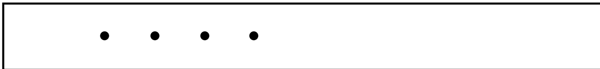
Example 4: Four 1/16 in. (1.6 mm) discontinuities
